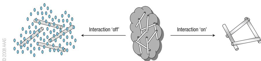
**Figure 2** A schematic representation of the polymer nanocomposite. In the 'on' state, interactions are formed between the cellulose nanofibres, which maximize stress transfer between the fibres and, as a result, the tensile modulus increases. These fibre–fibre interactions are removed by the addition of a biomedically relevant chemical that competitively forms hydrogen bonds with the fibres, and the system is switched to the 'off' state. Reprinted with permission from ref. 1.
