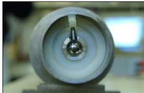
Front view of the bead sensor placed inside the ring holder.
