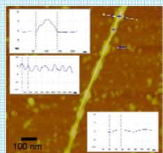
Figure 7: Air TMAFM; height image; AF with AuNP-CLPFFD on Mg<sup>2+</sup>-Ruby-Mica Z scan 1  $\mu$ m; Z range 15 nm; 512 pixels; E scanner; Superior section; horizontal distance: 70 nm; Middle section; horizontal distance 101 nm; Low section; vertical distance 1.335 nm
