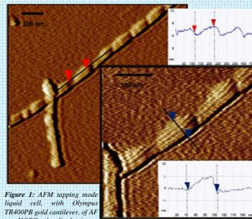
Figure 1: AFM tapping mode liquid-cell, with Olympus TR400PB gold cantilever, of AF on HOPG. Amplitude image and topography - Z scan 1  $\mu$ m and 400 nm; Z range 0.100 V; PF-scanner
