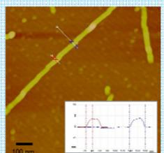
Figure 8: TMAFM Height image, AF on Mg<sup>2+</sup>-Ruby-Mica; Z scan 1  $\mu$ m; Z range 15 nm; 512 pixels; E scanner; Red section; vertical distance: 3.9 nm; Blue section; horizontal distance: 43 nm
