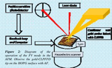
Figure 2: Diagram of the operation of the FV mode in the AFM. Observe the gold-CLPFFD tip on the HOPG surface with AF.
