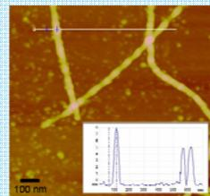
Figure 6: Air TMAFM Height image; AF with AuNP-CLPFFD on Mg<sup>2+</sup>-Ruby-Mica Z scan 1  $\mu$ m; Z range 15 nm; 512 pixels; E scanner; Superior section; horizontal distance: 70 nm; Middle section; horizontal distance 101 nm; Low section; vertical distance 1.335 nm
