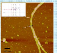
Figure 9: TMAFM Height image, AF on Mg<sup>2+</sup>-Ruby-Mica; Z scan 1  $\mu$ m; Z range 15 nm; 512 pixels; E scanner; Red section; vertical distance: 3.5 nm; Blue section; horizontal distance: 47 nm
